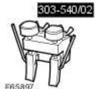
Tappet hold-down tool adaptor 303-540/02
